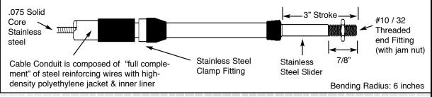
**PREMIUM** — PREMIUM Marine Cables are suitable for most applications where the control lever forces are between 20 and 40 lbs, and where the cable route is over 30 feet [10 meters]. PREMIUM cables can also be used in shorter applications where a smoother and easier control operation is desired.
