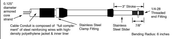
**EXTRA HEAVY-DUTY** — EXTRA HEAVY-DUTY Marine Cables are used in applications where the control lever forces are over 80 lbs.
