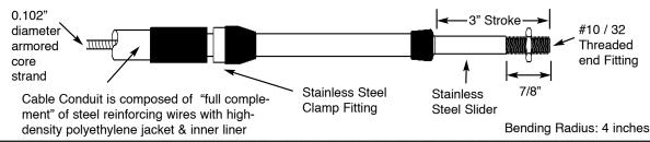
**HEAVY-DUTY** — HEAVY-DUTY Marine Cables are used in applications where the control lever forces are between 40 and 80 lbs.
