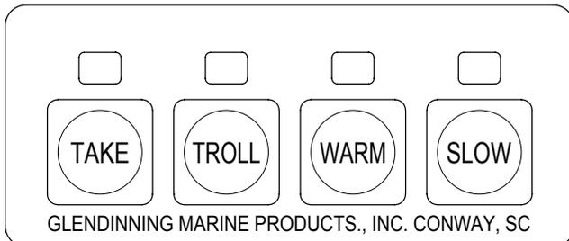
The CAT keypad is provided on boats equipped with electronically controlled diesels. Troll valve operation is activated by pressing the second button from the left.
