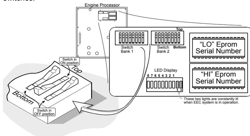
3. Position the DIP Switches as indicated below:
