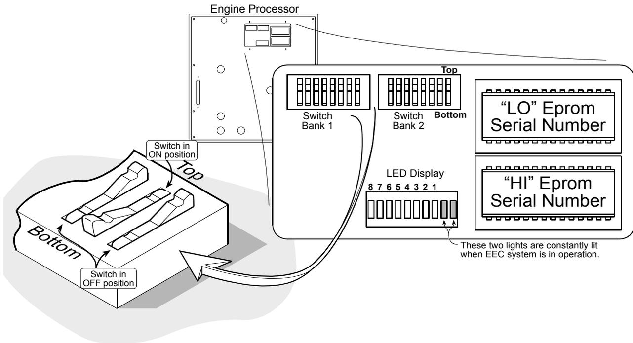
NOTE: To set the switch position, push down on the side of the switch that is marked with your desired setting. Example, **Push down on the OFF side** if you want the **switch to be in the OFF position**.
