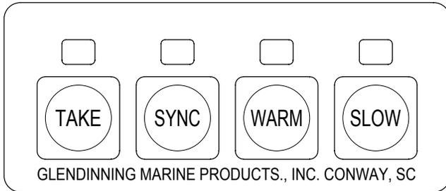
The Standard keypad is provided on boats not equipped with troll valves, and with non-electronically controlled diesels. Troll valve operation is not available with the standard keypad.
