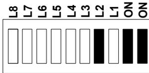
Starboard throttle calibration
