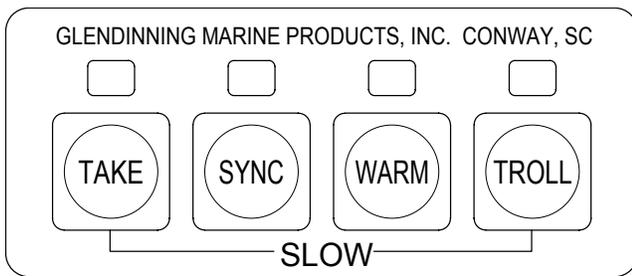
The Troll keypad is provided on boats equipped with troll valves, and with non-electronically controlled diesels. SLOW mode operation is activated with a “2-button” press (TAKE and TROLL buttons pressed simultaneously)
